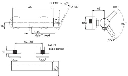
Work water pressure: Min.0.5kgf / cm²/ Max.5kgf / cm². (Including cold and hot.)
